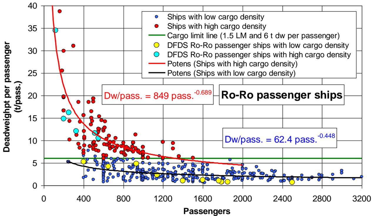
In addition to the cargo density class it is possible to change the maximum deadweight per lanemeter either in direct values or in percentage. Especially when the high cargo density type is chosen or when the dw/lanemeter is increased, it will be natural to change the ratio of payload in pct. of the deadweight from a default value of 55 – 60 pct. to 65 – 80 pct. as shown on the following figure.
