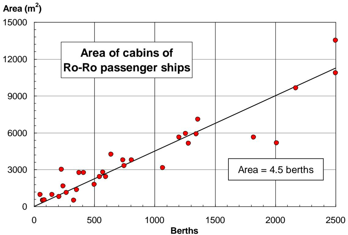
Fig. B4 Area of passenger cabins of Ro-Ro passenger ships (Hagemeister thesis work 2011)
